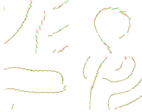
Figure 3. The edge orientations computed using the third-order orientation operator, Equation 3, (shown in green) compared to those obtained from the gradient of the image (shown in red). That the results are dramatically better is evidenced by the self consistency of edge orientations as one travels along each curve, as opposed to the red edges which deviate significantly from the curve tangent.
